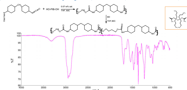
Fig. 7. Reactivity test of HO-PIB-OH towards 4,4'-diisocyanatodicyclohexylmethan (H 12 MDI).
